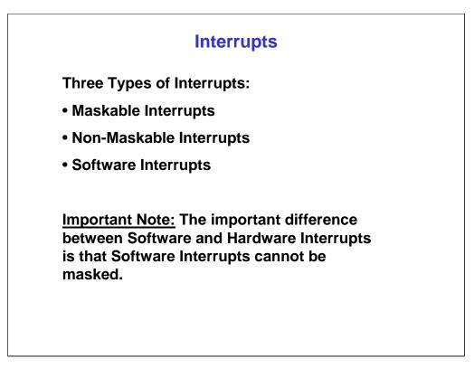
Now that we have discussed different types of reset sources, let's move on to interrupts and their various sources. There are three types of interrupts: Maskable, Non-Maskable, and Software Interrupts. When an interrupt event is detected, the MCU temporarily suspends the current program execution, which allows the MCU to service the interrupt request.
