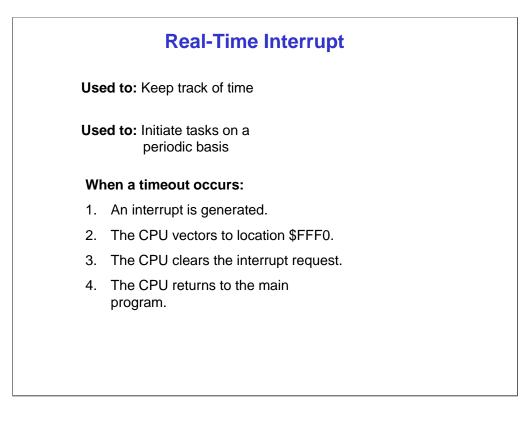
Now, let's take a look at Real-Time Interrupts (RTIs). RTIs are used to keep track of time and to initiate tasks on a periodic basis. When a timeout occurs, an interrupt request to the CPU is generated and the RTI vector is fetched from address (\$FFF0).
