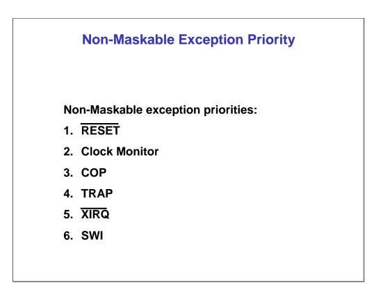
It is important to note that there are over 50 interrupt sources and each reset or interrupt source has a separate vector.
