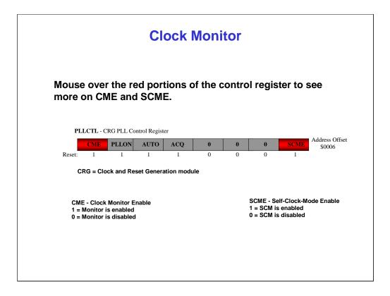
The Clock Monitor and the SCM are enabled out of reset. This allows the MCU to run from the internal RC oscillator if the crystal clock is not present. The internal RC clock ranges from one to 5.5 MHz.
