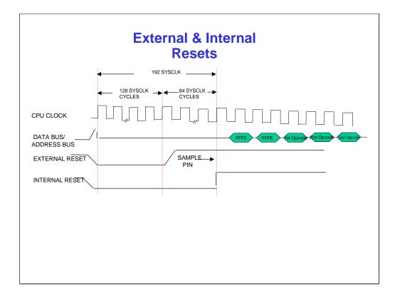
The address bus is driven with the appropriate vector address upon reset, whereas the data bus is used to read the contents of the vector and places it in the program counter to invoke the reset handler. The MCU reads 3 opcodes from the reset handler before instruction execution is started. Since the HCS12 family has 3 stage instruction queue, the queue has to be filled by executing three read operations".
