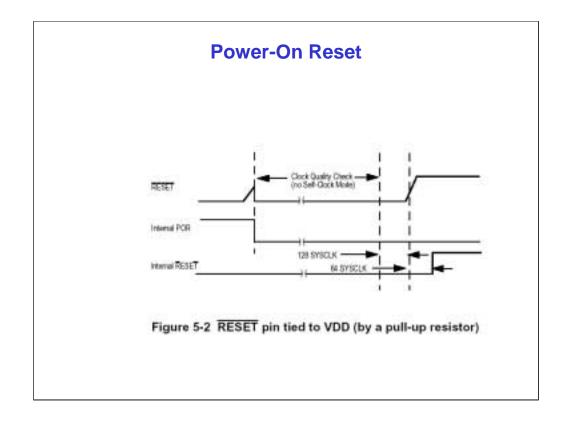
Let's take a look at Power-On Reset in more detail. Power-On Reset is initiated by positive transition on VDD. A Clock Quality Check begins after the Power-On-Reset (POR) trigger. The reset pin is tied to the VDD by a pull-up resistor.
