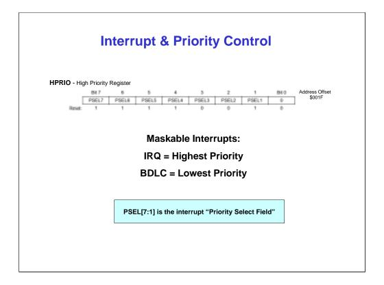
A maskable interrupt source can be elevated to the highest priority by writing to the High Priority (HPRIO) register, bits 7 to 1. Interrupt priority can only be changed when I-bit is set to a '1' in the Condition Code Register, CCR.
