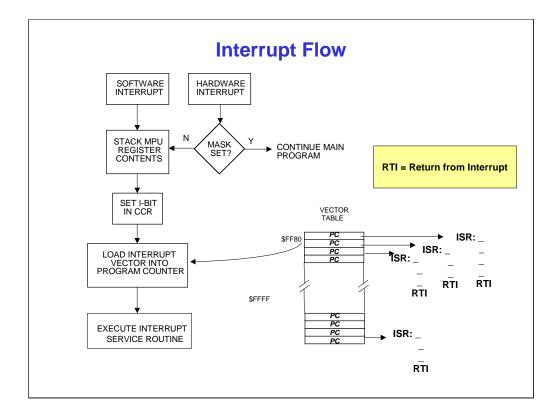
When the CPU receives an interrupt request, it first completes the current instruction being executed. The CPU also pushes all CPU registers onto the system stack in order to remember the previous state of the machine. The CPU then updates the CCR to mask out further interrupts. The interrupt event causes the MCU to vector to one of the many in the vector table in order to point to the appropriate service routine.
