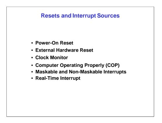
Resets and interrupts are responses to exceptional events during program execution. Six reset and interrupt sources include: Power-On Reset, External Hardware Reset, Clock Monitor, Computer Operating Properly (COP), Maskable and Non-Maskable Interrupts, and Real-Time Interrupts.
