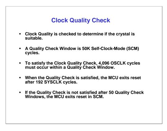
The Clock Quality is checked to determine if the crystal is suitable to run from when POR occurs, when exiting STOP mode, and/or after Clock Monitor failure.
