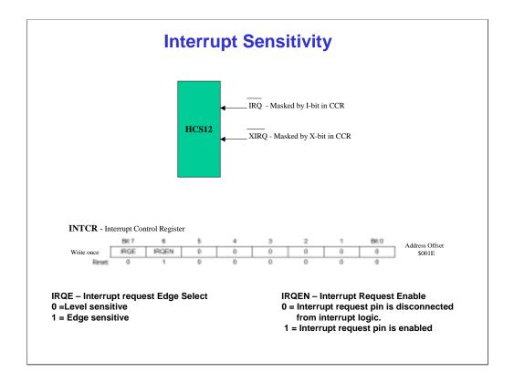
The HCS12 has two external pins called IRQ and XIRQ. The IRQ pin generates Maskable Interrupts, while the XIRQ pin generates Non-Maskable Interrupts. Here, you can see that the IRQ pin is masked by the I-bit in the CCR, and the XIRQ interrupt is masked by the X-bit in the CCR. When the XIRQ interrupt is enabled, it cannot be disabled and becomes a nonmaskable interrupt source.
